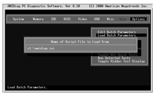
Press Enter to accept the default batch parameter file (Diagnostic Utility.INI), or type the appropriate AMIDiag batch parameter filename. You can use any valid filename.
